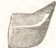
For Wrought Iron, where Tool is Liable to Spring on account of Distance from Tool Post.
