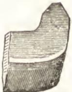
For Cast Iron, where Tool is Liable to Vibrate, or Tremble.
