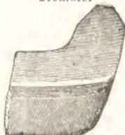
For Cast Iron, The Back Part is for Scraping; the Front Corner is for Cutting.
